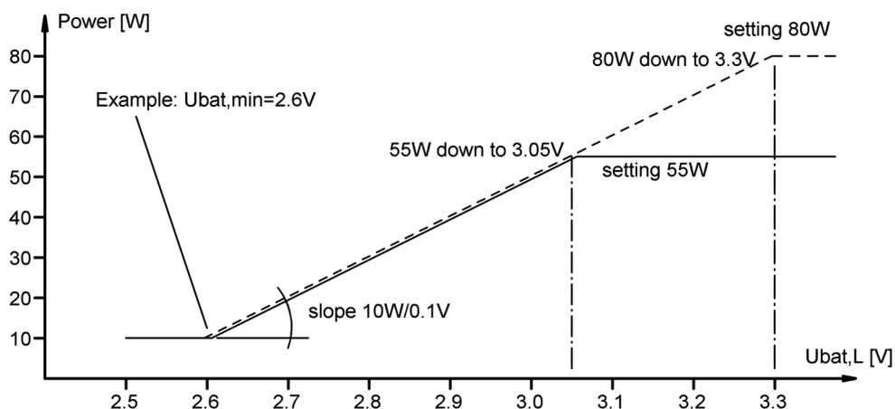
At  $U_{bat,Min} + 0.7V$  a power reduction is activated depending on the actual power setting. The reduction starts when the power selected hits the slope from  $U_{bat,min}@10W$  to  $U_{bat,min}+0.7V@80W$  as show in the diagram above.
